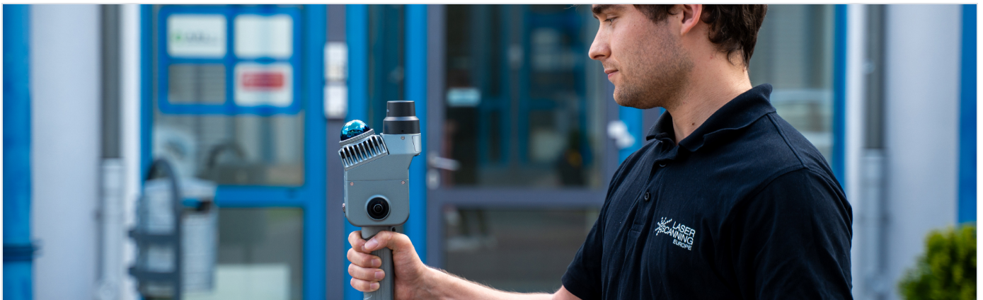
The sideways threshold: walk the opening so the scanner sees both sides at once
