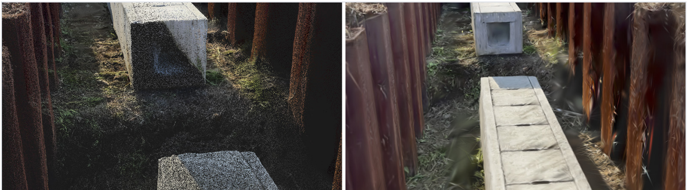
One capture, two deliverables: point cloud (left) and 3DGS splat scene (right) of the same trench
